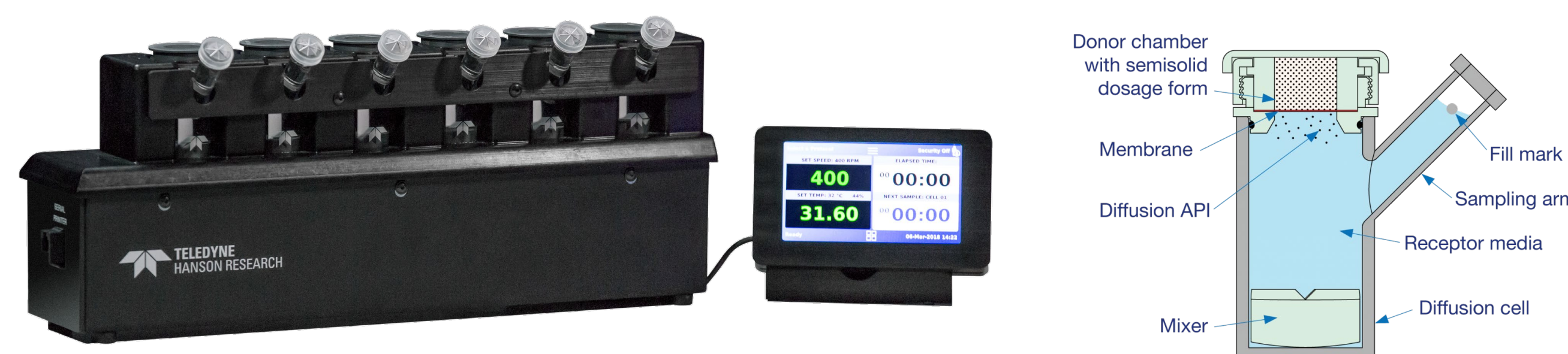
Figure 1. Phoenix DB6 from Teledyne Hanson and schematic of Diffusion cell.
