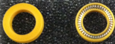
Figure 8, Example of polymer side vs. energizer side of seal. Note: stainless steel energizer shown. Seal could have fluoropolymer o-ring energizer instead (black o-ring).
