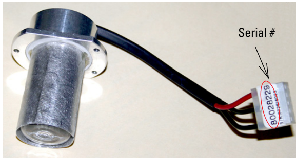
Figure 6: Removing lamp from bracket
