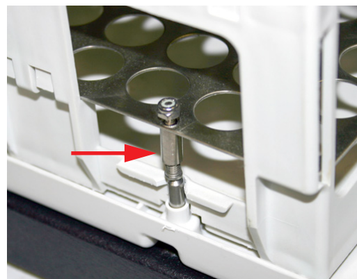
Figure 8: Rack grounding pin function
