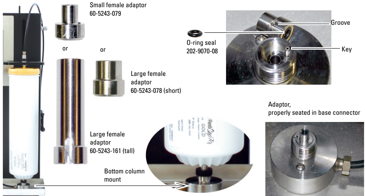
Figure 33: Installation of bottom column adaptor and o-ring
