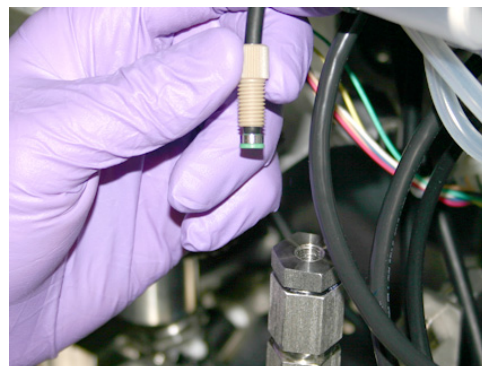
Figure 27: Disconnect tubing from filter assembly
