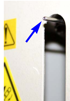
Close-up view of nitrogen purge tube (This view applies to pumps other than the 1000D)
