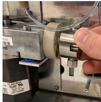
Figure 7: Reinstalling the pump head
