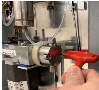
Figure 8: Reinstalling the fasteners
