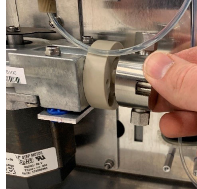
Figure 3: Removing the pump head
