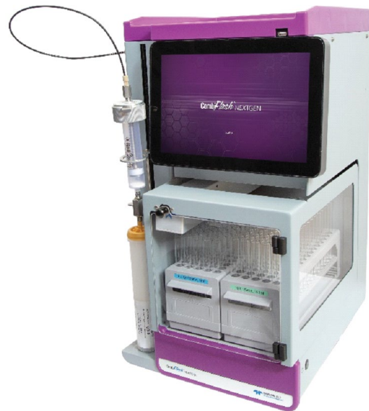
Figure 9. Secure the cartridge assembly on the system (CombiFlash NextGen shown).
