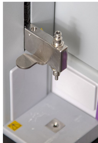
Figure 1. Injection port trolley.
