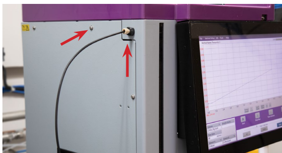
Figure 3. Left instrument panel screw and liquid port locations.
