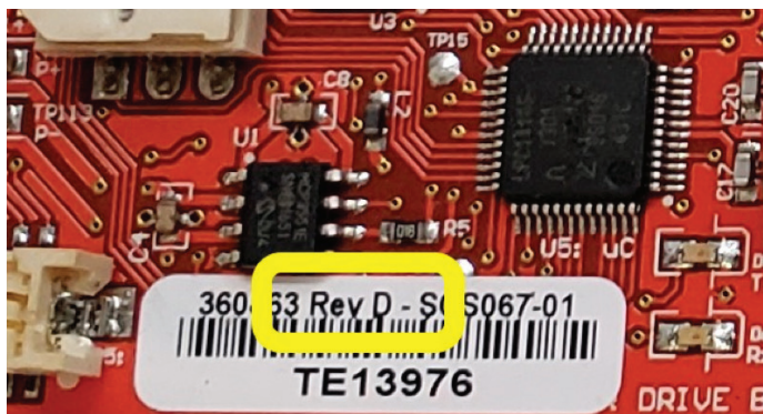
Figure 18: Pump board revision sticker
