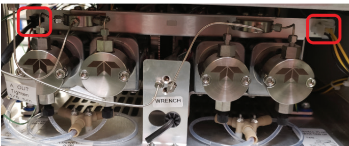
Figure 3: Pump assembly electrical connection locations
