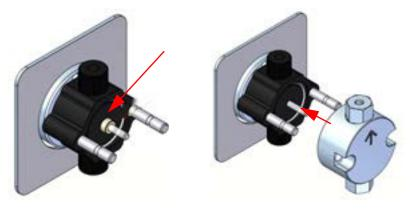
Figure 5-16 Reinstalling the pump head
