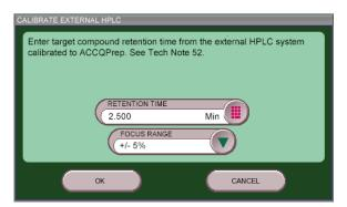
Figure 2-12 The HPLC Focus window
