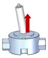
Figure 5-12 Removing the seals
