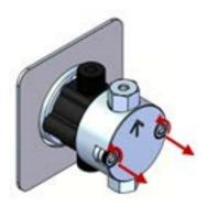
Figure 5-9 Removing the fasteners
