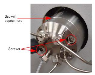
Figure 5-5 Location of the stator retaining screws
