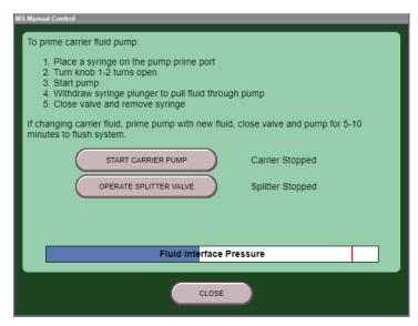
Figure 4-21 Mass Spectrometer Manual Control window
