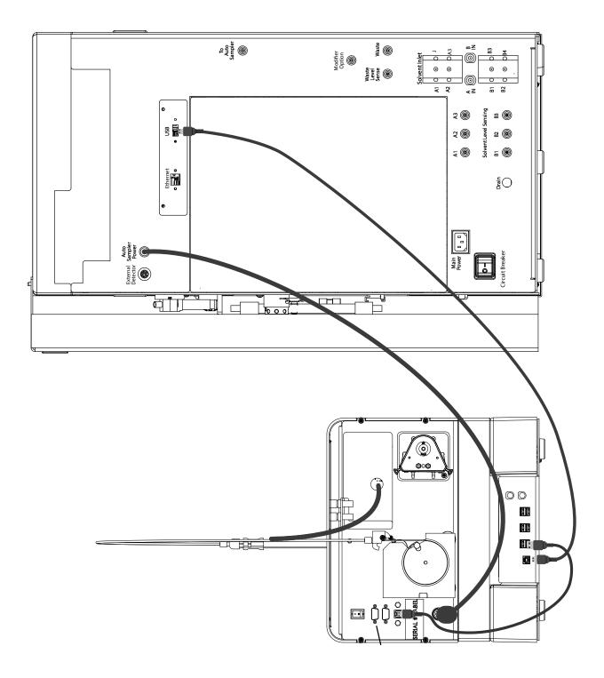
Figure A-2 Wiring diagram
