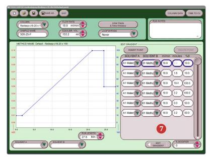
Figure 4-9 Method Editor screen with Edit Gradient panel
