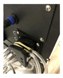
Figure 5-28 Attaching the new tubing
