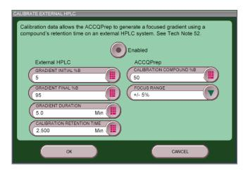
Figure 2-11 The Calibrate External HPLC window
