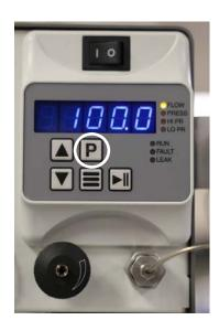
Figure 3-4 Loading Pump P button
