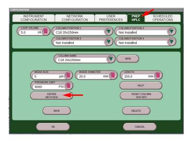
Figure 2-5 Column Configuration
