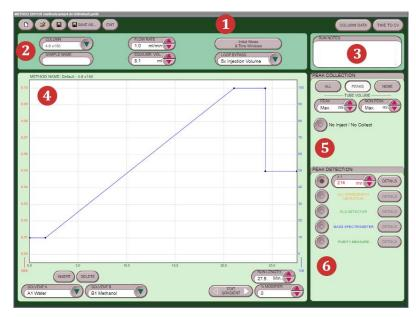
Figure 4-8 Method Editor screen with Peak Collector and Peak Detector panels
