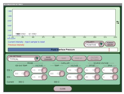
Figure 4-22 Mass Spectrometer Ionization Settings window
