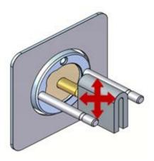
Figure 5-13 Cleaning the piston
