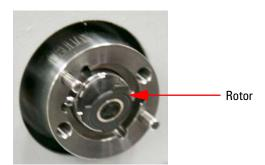
Figure 5-6 Removing the rotor
