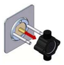
Figure 5-11 Removing the pump spacer block
