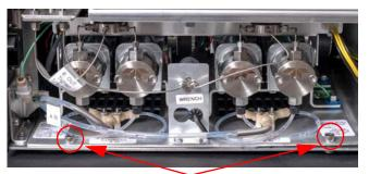
Pump assembly mounting screws
