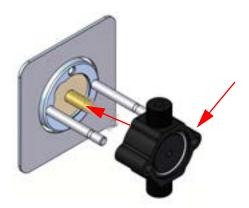
Figure 5-15 Reinstalling the pump spacer block
