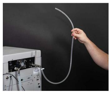
Figure 5-31 Line filled with 40 mL of acetone
