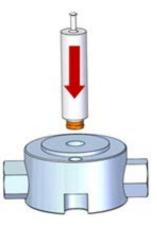
Figure 5-14 Replacing the seal
