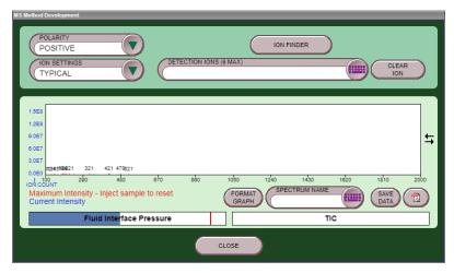
Figure 4-19 Mass Spectrometer Method Development window
