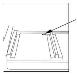
Vacuum or pressurized air applied to the outlet end of the drain tube must be present at the collection tray drain hole.
