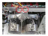
Figure 5-23 Location of tee mounting screws
