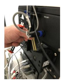
Figure 5-27 Removing the tubing
