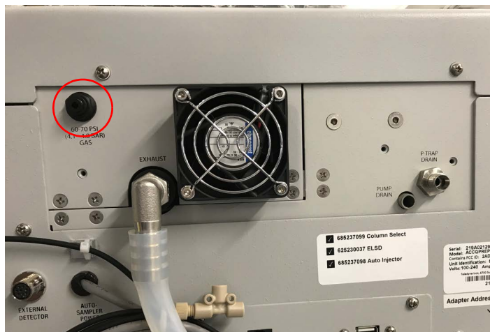
Figure 2-9 Location of ELSD gas port (Nitrogen input line circled)
