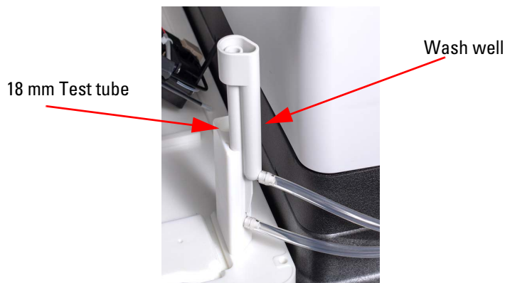
Figure 2-27 Location of the test tube and the wash well on the AutoSampler
