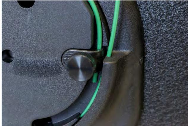
**Figure 3-9** Cable Installed on Rotor
