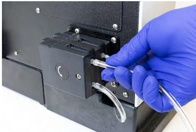
**Figure 3-23** Connecting the Rinse Solution Source to the Pump
