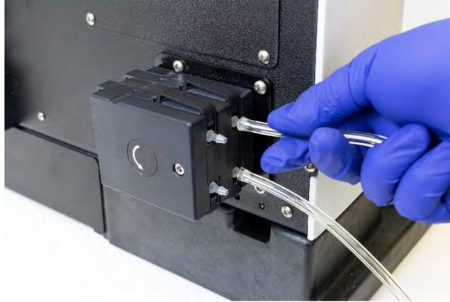
**Figure 3-16** Connecting the Rinse Station Drain to the Pump Input
