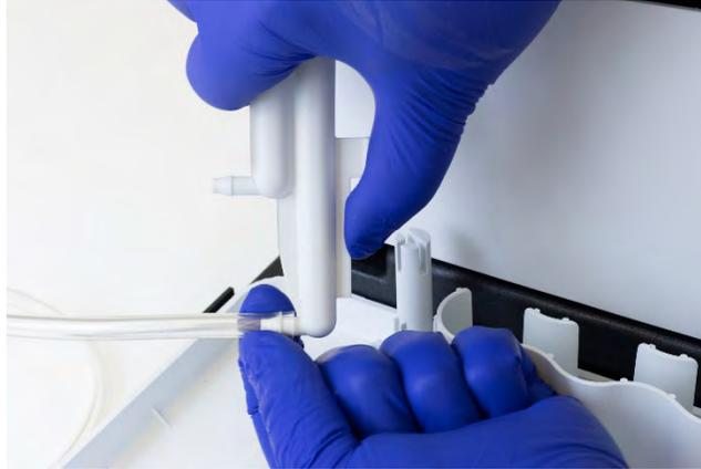
**Figure 3-20** Connecting Tubing to the Rinse Station
