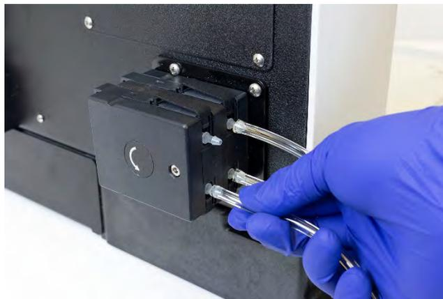
**Figure 3-17** Connecting the Pump to the Rinse Station Inlet
