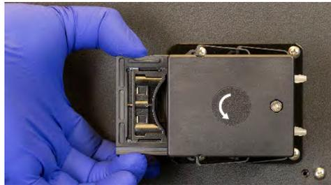
**Figure 7-7** Removing the Peristaltic Pump Pressure Shoe
