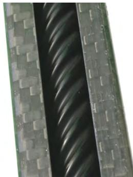
**Figure 7-1** Y-Axis Lead Screw
