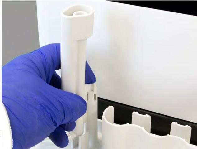
**Figure 3-1** Mounting the Rinse Station
