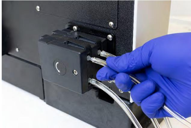
**Figure 3-18** Connecting the Rinse Solution Source to the Pump
