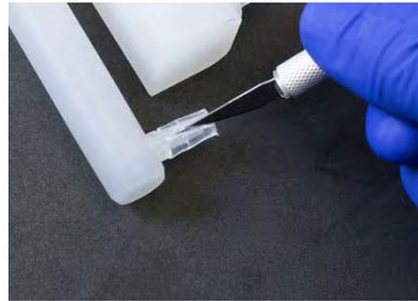
**Figure 7-3** Removing Tubing from the Fitting
