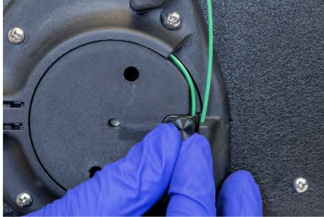
**Figure 3-8** Securing Cable to Rotor
