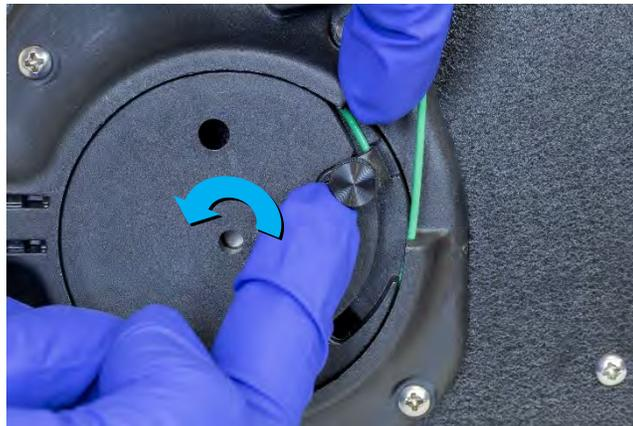
**Figure 3-7** Position of Cable on Rotor
