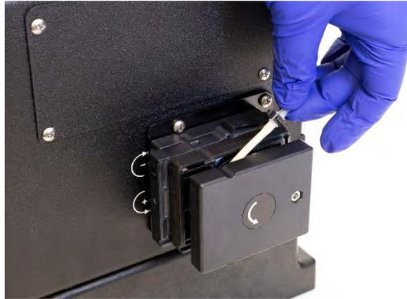
**Figure 7-8** Removing the Peristaltic Pump Tube
