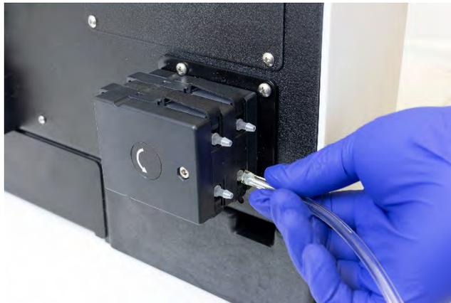
**Figure 3-15** Connecting the Waste Line
