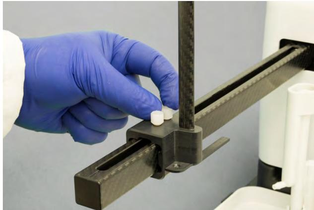
**Figure 3-5** Securing Z-Drive Onto the Arm
