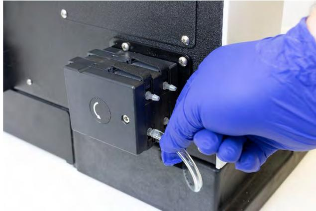
**Figure 3-22** Connecting the Pump Output
