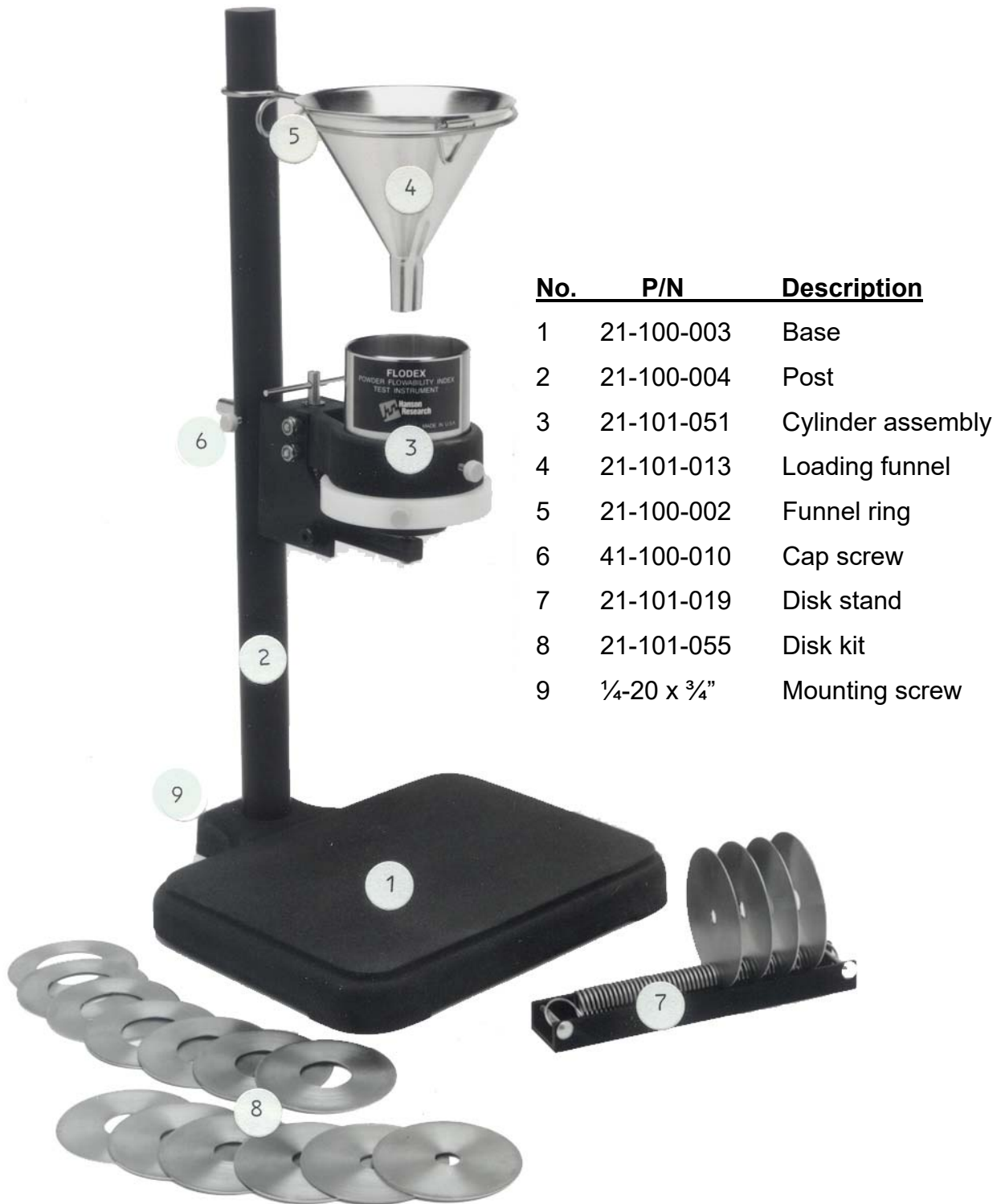
Figure 1 – Flodex final assembly (p/n 21-101-050)
