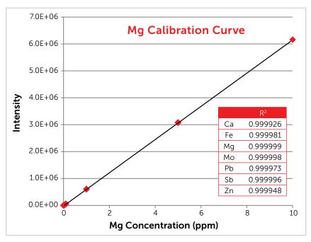
**Standard Preparations** – The SimPrep can prepare the entire curve from a single stock solution. This brings a high level of precision and accuracy to the most important prep of the day. Don't worry about the analyst on duty or the day of the week - get the same prep every time. Autocalibration data from a 6 point curve. Standards prepared from a 100 ppm stock at  $10 \times to$   $2000 \times dilution$ .
