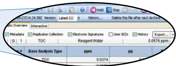
Sample History, Electronic Signatures, Metadata, Replicates Collection and User IDs are some options you can choose with the exporting data function.
