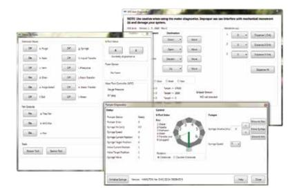
**Diagnostics Options** - Direct control of system components along with automated Benchmark Test validation and System Leak Check. Maintenance wizards assist in syringe replacement/initialization and autosampler alignment.
