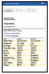
Instrument Status Screen -Provides real-time monitoring of the analytical process including active method, current mode and a complete list of current instrument parameters and their set points.
