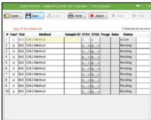
**Schedule Screen** - Schedule building is easier than ever thanks to excel-based features such as highlight, fill down and fill sequential commands. Schedules can be edited at any time, even while running. This allows for priority samples to be added in at any time. Schedule screen also includes useful fields such as sample ID, Internal standards addition, and vial position. Lastly, the schedule captures essential information such as purge and bake pressures, and sample status.
