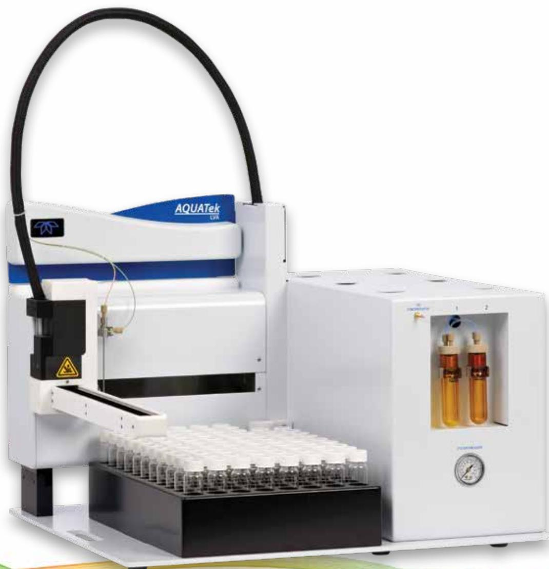
The AQUATek LVA automates the sample preparation steps for the analysis of liquid samples via purge and trap. The system is capable of preparing samples such as drinking water and wastewater. With intuitive self-diagnostics and user-friendly software, the AQUATek LVA is the simplest, yet most robust autosampler on the market today.
