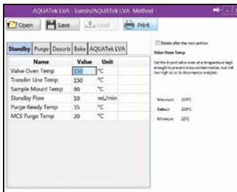
**Method Development Screen** - The Lumin TekLink™ software comes pre-installed with methods for most applications. You can select one of these methods or if your application calls for a unique requirement, a customized method can be created to meet your analytical requirements for sample processing.
