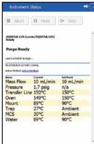
**Instrument Status Screen** - The Instrument Status screen provides valuable information such as mode of operation and instrument conditions. During Leak Check, it displays the region of the system that is being checked and the time remaining of the leak check.
