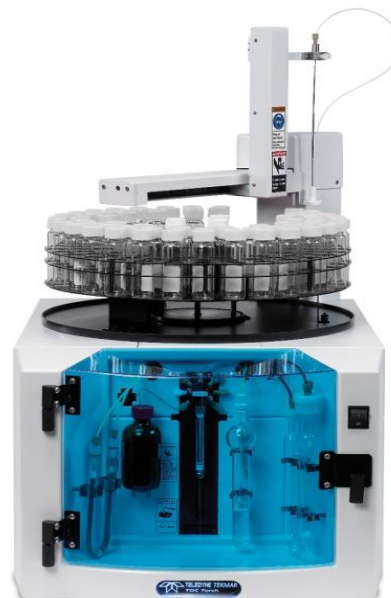
Figure 3 Torch Combustion TOC Analyzer
