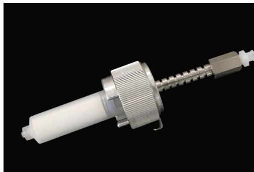
Figure 5: Silica solid load cartridge and cap with a Luer adapter.
