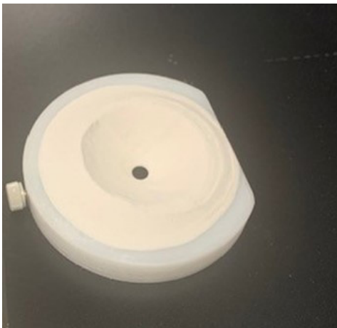
Image 2: Appearance of a successful powder flow test (part of cylinder removed for clarity).
